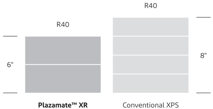
**Plazamate™ XR gives designers and builders maximum Styrofoam™ insulation performance with minimum thickness.**
