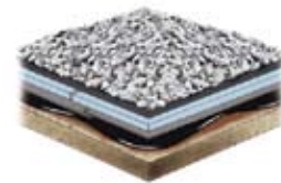
Protected Membrane Roof
